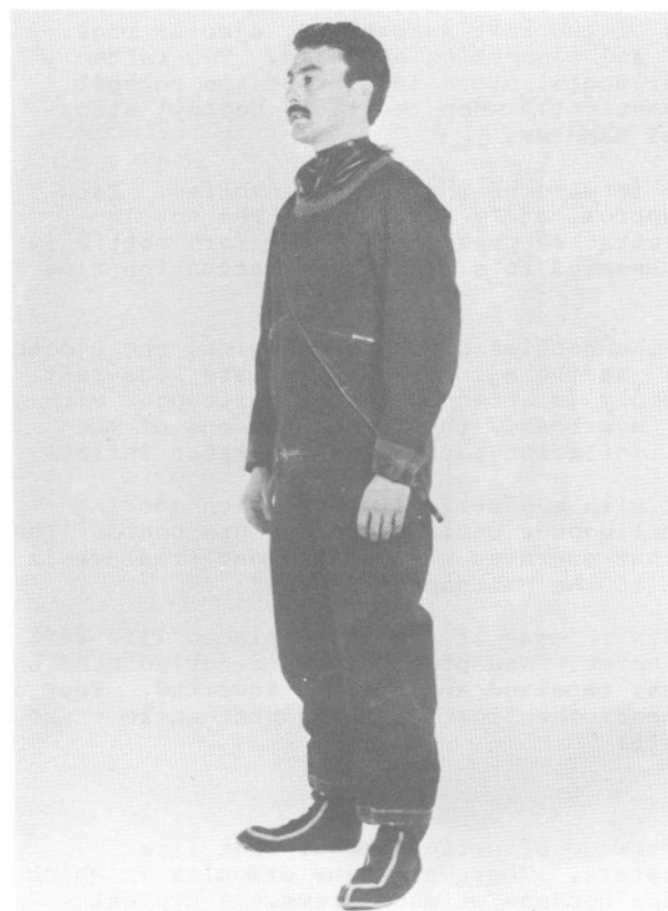
C. RAF upper half single layered cotton ventilate suit for NBC conditions. - Diagonal zip. (Courtesy Dunlop - Beaufort Ltd.)
